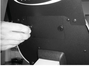
Use coin to remove battery access panel.
